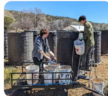
Heather Hillyer and Mathew Chavez using muscle power to lift buckets of combined food and shredded wood into the modified bioreactor. Photo by Carol Ann Fugagli
