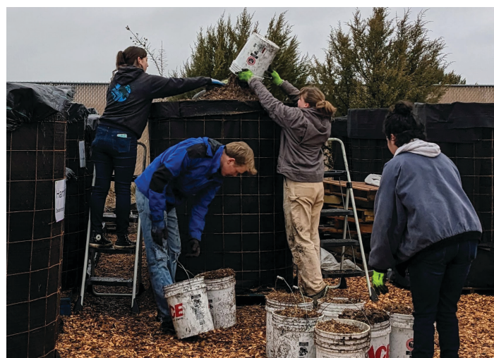
Zoe Pitts, Colin Casler, Molly Pendleton, and Rachel Gulick, filling a bioreactor with combined food slurry and shredded woody biomass. Each bioreactor contains approximately 1,800 pounds of feedstock. Photo by Carol Ann Fugagli
